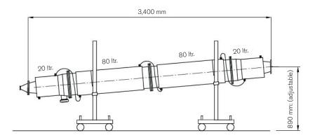
The GS resting tube is delivered with strainers, standard inlet cone, and is mounted on a frame. Pneumatic 3-ways valve can be supplied.
